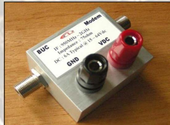
This small and efficient unit provides DC supply to a BUC (DC power supply separate) in case a modem cannot supply sufficient power or doesn't provide BUC power at all. The unit passes L-Band signal and 10MHz reference signal and injects up to 6A DC current.
